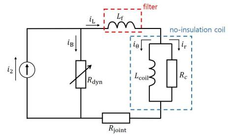
Keywords: charging performance, filter inductor, flux pump, no-insulation REEBCO pancake coil
