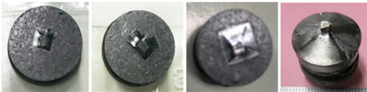
Figure 1. As grown bulk Y-123 superconductors produced by Top Seeded Infiltration Growth Process utilizing a mixture of Yb-123+liquid phase as a liquid source in 50 hours. Yb-123+liquid (1:1) left; Yb 123+liquid (1:1.2) middle left; Yb-123+liquid (1:1.3) middle right; Yb-123+liquid (1:1.3) right (> 50h)
